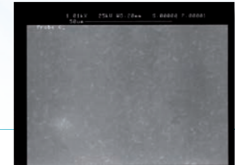
REM IMAGE OF A STANDARD VENTRICULAR CATHETER, TYPICALLY OF SILICONE
